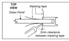
provided to remove the excess silicon. Remove the masking tape immediately after application.
