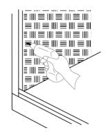
**6.** Apply a continuous bead of silicon to the full length of the channels and waterproofing, indicated by the dark line (inside channel).
