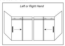
2. Position glass receiver channel over the base glazing channels. Use a straight edge and mark the wall to indicate where the wall channel is plumb.
