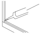
Ensure the corner junction between wall channel and base channel is full of silicon before final glass
