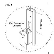
**8.** Apply plastic packers (bag11)into the base glazing channels in locations as shown.
