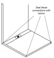
Prior to installation of glass panels and infill all connections of channels, must be sealed with clear silicon supplied
