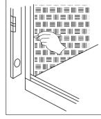
**3.** Apply a silicon seal to full length of channels. Silicon used must be compatible with anodised aluminium as well as the waterproofing being used.
