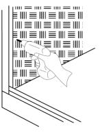
6. Apply a continuous bead of silicon to the full length of the channel and waterproofing, indicated by the dark line (inside channel).
