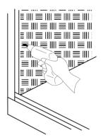
5. Apply a continuous bead of white silicon to the full length of the channels and waterproofing membrane, indicated by the dark line (inside chan
