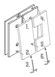
Fit the hinges, the removable cover must be on the outside of the shower.
