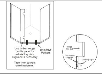
ENSURE HINGES ARE CLEAR FROM SIDES OF GLASS CUTOUTS AND HINGE BOLTS ARE FINALLY TIGHTENED AS MUCH AS POSSIBLE.
