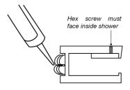
4. Ensure the glass receiver channels are located firmly over the base glazing channels. Locate the framing timber. Use the 4mm drill bit to drill holes through the glass receiver channels. Fix four screws through the channels into the wall framing (use wall plugs if required supplied with wall channels).
