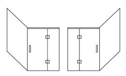
Position the glass receiver channels over the base glazing channels. Mark the wall to indicate where the wall channels are plumb.
