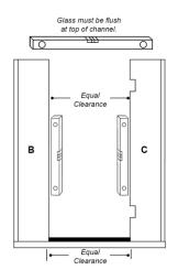
glazing channels. The top of the panels should align to the top of the glass receiver channels. Add or remove packers in the base glazing channel as
