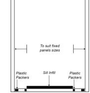
shown. Sill infill must measure 3mm larger than door, trim if required.
