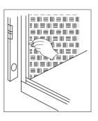
Apply a silicon seal to full length of channel. Silicon used must be compatible
