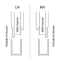
5. Locate the framing timber. Use the 4mm drill bit to drill holes through the glass receiver channels. Fix four screws through the channels into the wall framing (use wall plugs if required).
